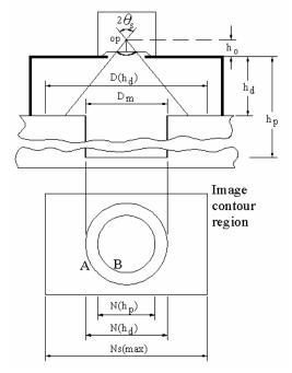
Fig. 4 Schematic diagram of measurement frame.
