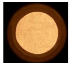
Hole-diameter of sample: 22mm Hole-depth of sample: 14.9mm Fig. 2 actual image contour region of sample I
